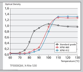
KPW 490, KPW 415, KPW 417, KPW 421 and KPW 423 are, in terms of static sensitivity, equivalent to KPW 412.
